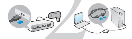
**TIP:** A half-hitch knot helps ensure USB extension cables stay linked together. Ensure that the USB device has no more than 15ft of cable between it and the nearest USB hub.
